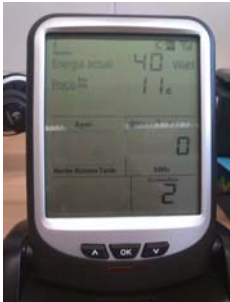
Figura 3: Smart meter (Current Cost)
